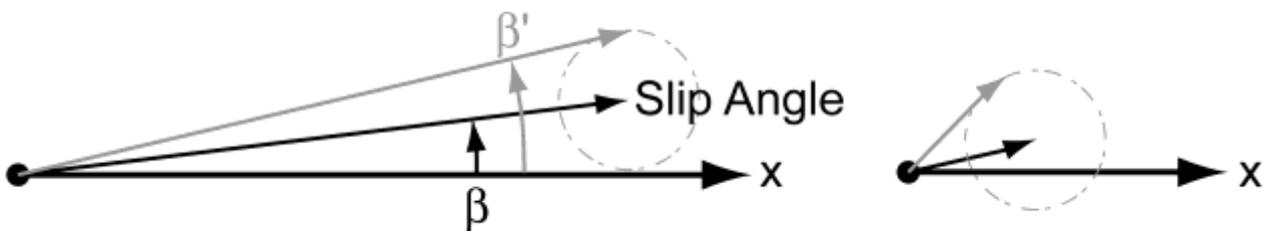
As the velocity line gets shorter (right) and the effect of the error on the slip angle increases; see how the same sized circle has caused the grey slip angle measurement to have a bigger difference compared to the true slip angle (black). The diagram on the right has a much shorter velocity error, but the reported slip angle (grey) has a bigger error on it compared to the diagram on the left.
