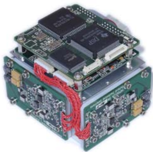
Inertial Sensors in RT3000 include servo-grade accelerometers and precision MEMS angular rate sensors. Powerful 40MHz floating point DSP takes care of coning, sculling and aliasing.
