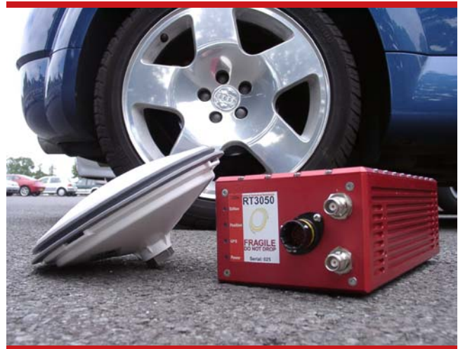
RT3050, OmniStar GPS Antenna with Integral Ground Plane
