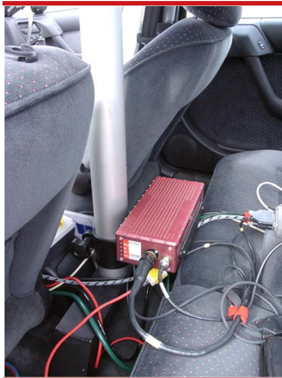
Figure 2. RT3100 Installed on Mounting Strut close to Centre of Gravity.
