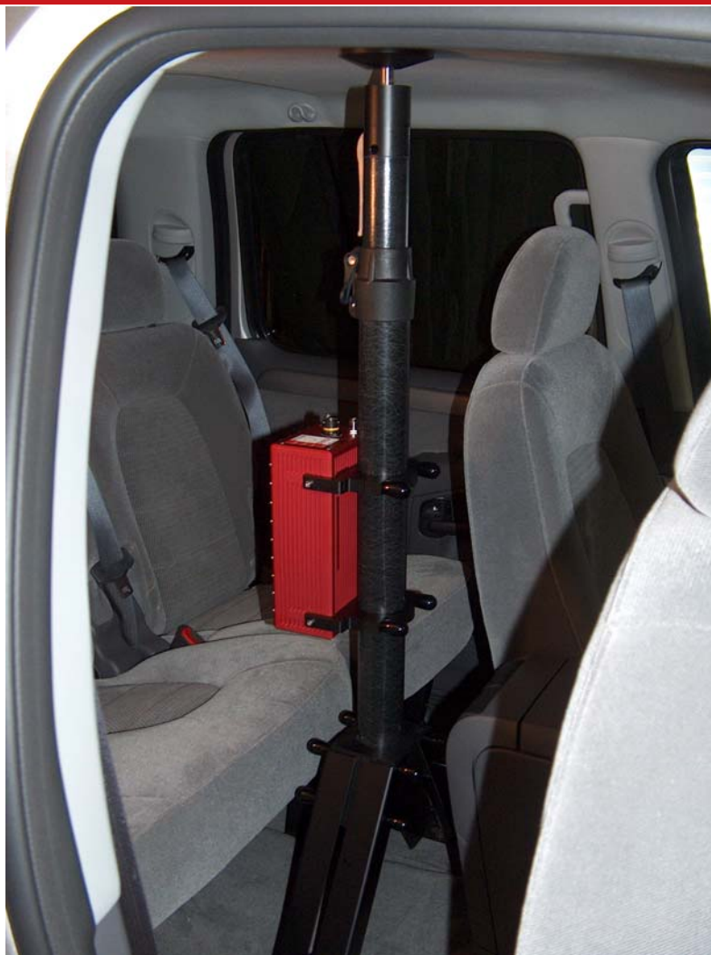
Figure 1. RT-Strut Mounted in a Car
