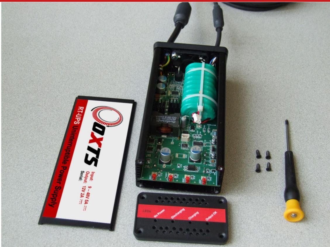
Connect the battery wires to the socket on the circuit board as shown in Figure 3. The connector can only be fitted one way round; take care not to force it incorrectly. Slide the lid back in place, fit the front panel and replace the four screws. The battery will now be connected correctly.
