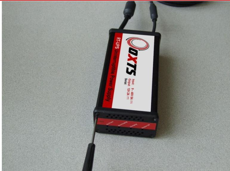
Remove the front panel and slide the lid off the RT-UPS, as shown in Figure 2.
