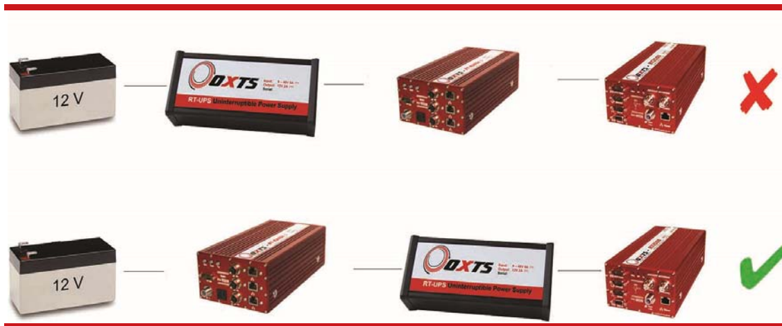
Figure 4. Connection set-up with RT-Range or RT-Range S
