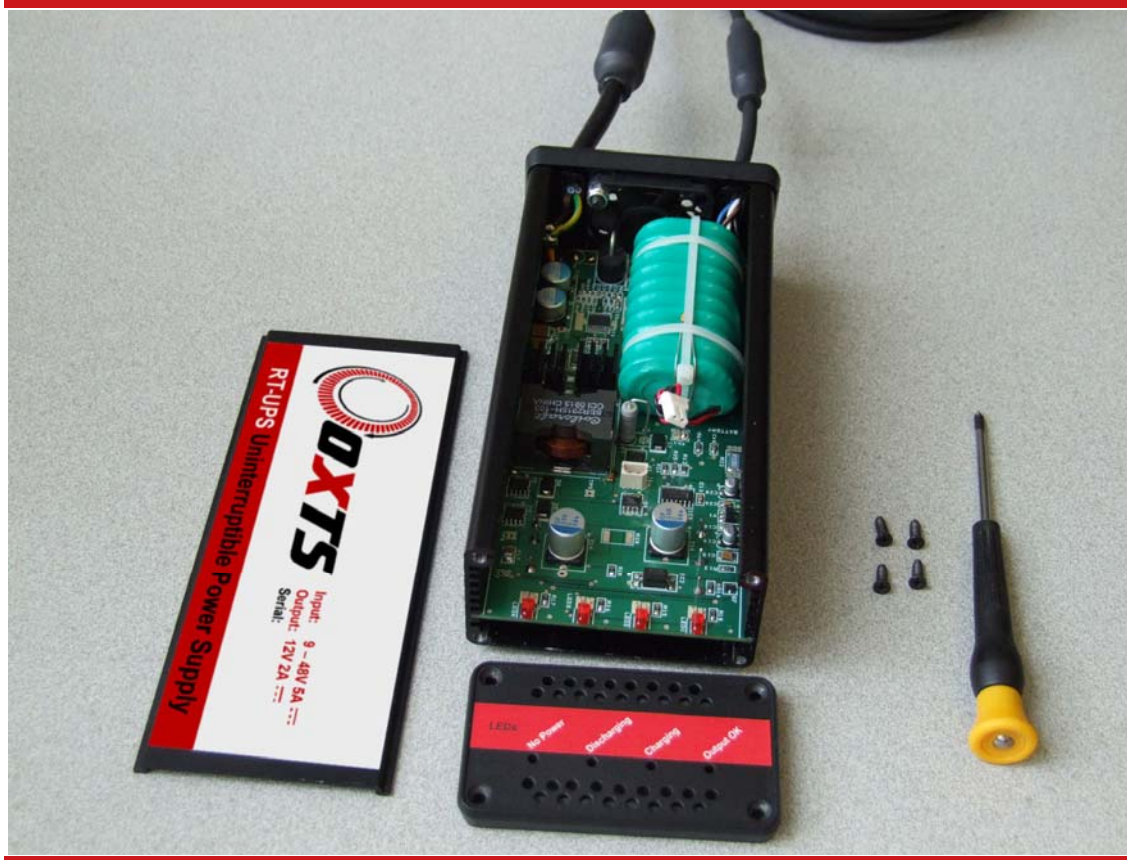
Figure 2. RT-UPS showing the battery connector
