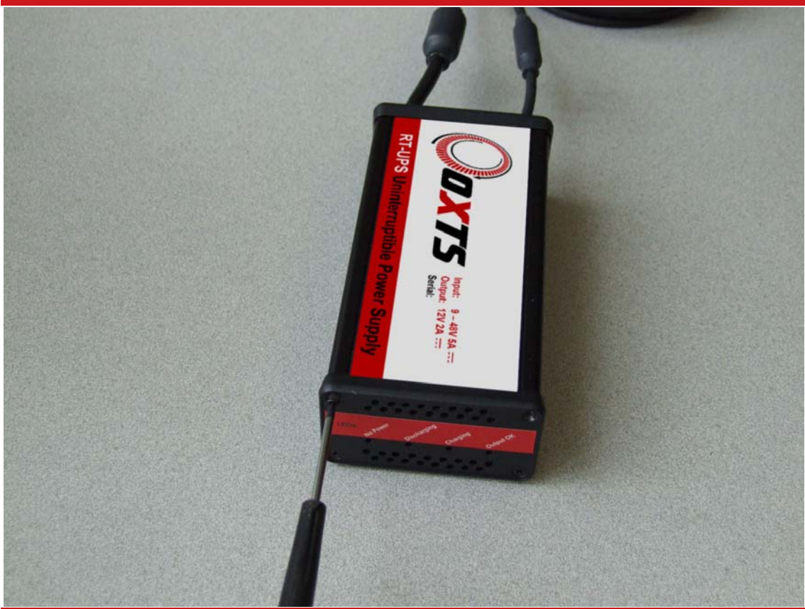
Figure 1. Removing the front panel screws on the older model RT-UPS
