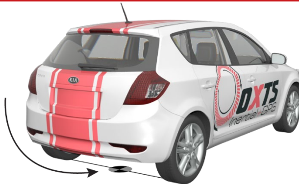
Figure 26. Measurement point for Advanced slip
