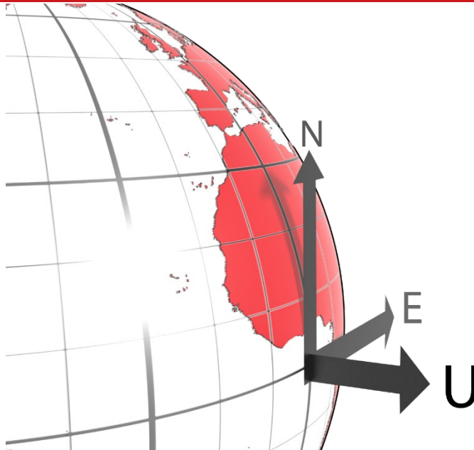
Figure 8. ISO 8855 ENU earth-fixed system
