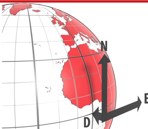
Figure 7. OxTS NED navigation frame definition
