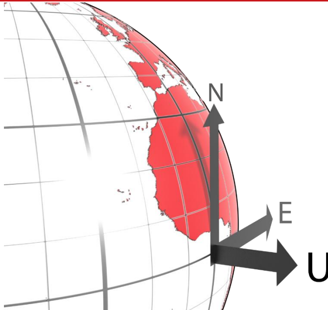
Figure 8. ISO 8855 ENU earth-fixed system
