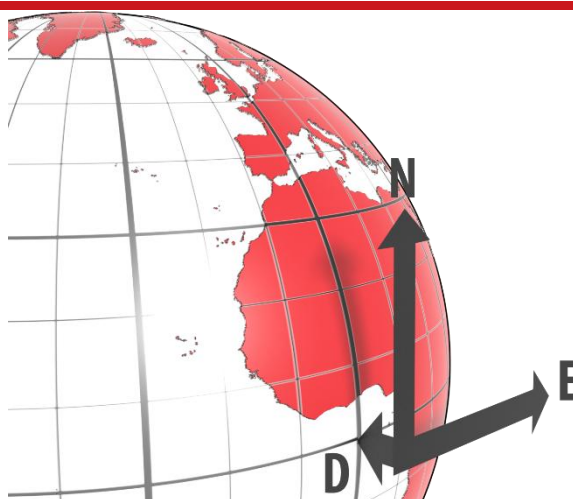
Figure 7. OxTS NED navigation frame definition
