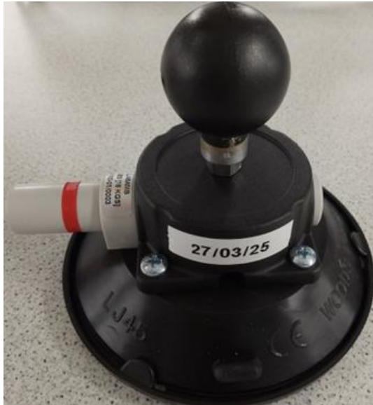
Figure 29: LiDAR roof mount suction cup inspection date
