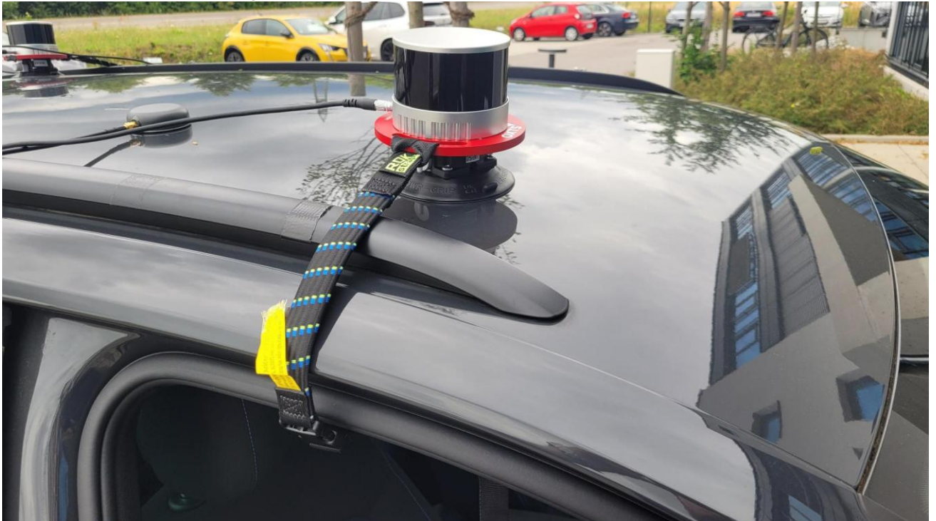
Figure 33: Retaining strap attached to LiDAR suction cup roof mount
