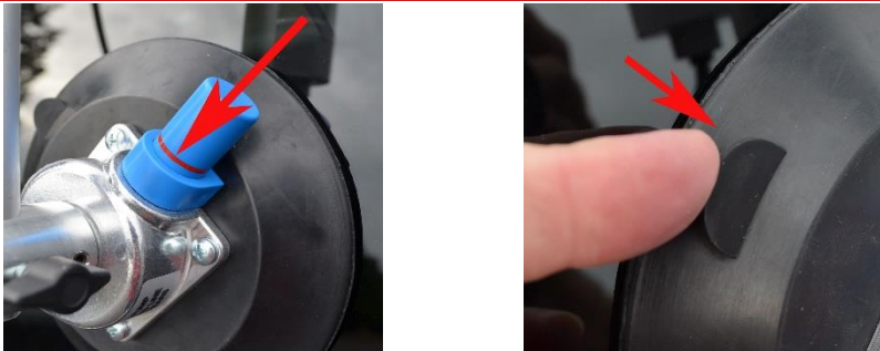
Figure 2. Attaching and removing the pump cup
