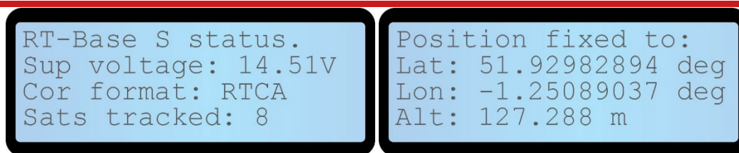
Figure 10. LCD status pages once position is fixed
