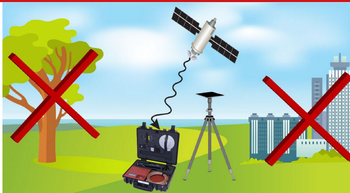
Figure 4. Choosing a location for the GNSS antenna
