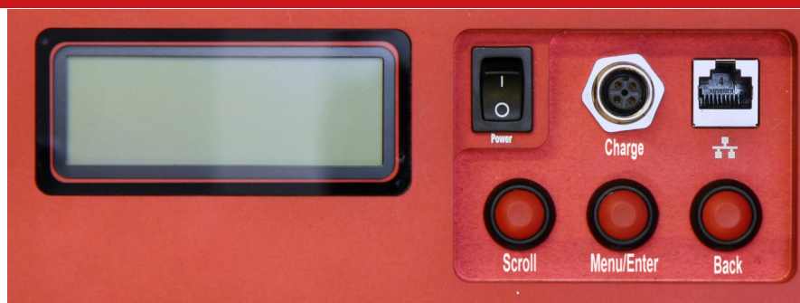
Figure 6. The control panel on the RT-Base S
